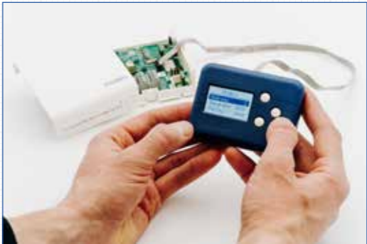
SIRO-CT ENABLES COMMISSIONING OF SIRO DEVICES WITHOUT DISPLAY
