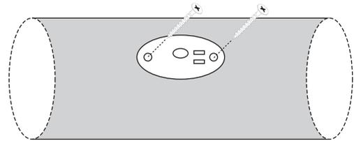
**Figure 1b - Mounting the probe in a flange**
