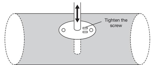
**Figure 1c - Mounting orientation**
