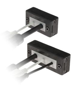
The DES L2 and L3 splittable frames enable pre-terminated cables from 2 to 16mm in diameter to pass through enclosure walls, providing strong strain relief and water protection.
