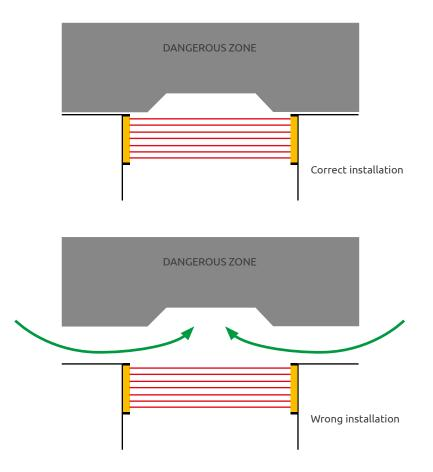
It shall not be possible to reach the dangerous area by climbing on the machine or crawling below the sensitive area or leaning over the edge of the sensitive area.
