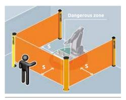
Fig. 14. Three-side protection using deflection mirrors
