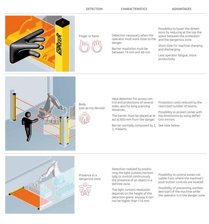
Accidental start-up of the machine shall not be possible when anyone crosses the sensitive area and stays undetected in the dangerous area. Suitable ways of eliminating this type of risk include the following: Use of start / restart-interlock function positioning the command so that the dangerous area is in full view and so that the command cannot be reached by anyone from inside the dangerous area. The Restart command has to be safe.
