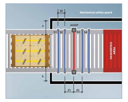
Muting with 2 crossed-beam or parallel-beam sensors – Configuration type L with timing monitoring and one-way only(exit from dangerous area) pallet operation:
