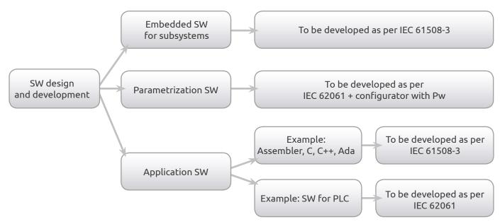
Safety-related PLCs, safety bus, actuators, safety light curtains and in general all complex safety-related devices with integral programmable logics and embedded software, if used to build a SRECS, shall comply with the requirements of the appropriate Product Standards (if applicable) and with IEC 61508 as regards functional safety.
