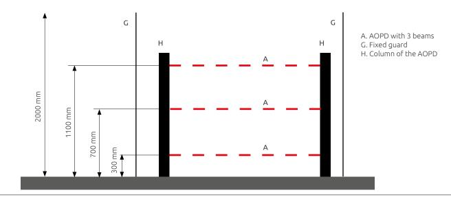
Fig. 23. Positioning of the AOPD - General
