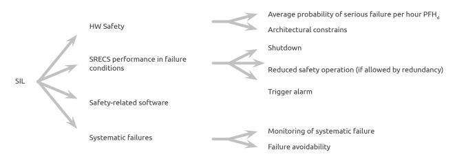
Each subsystem shall consist of electrical circuits suited to attain the required SIL.
