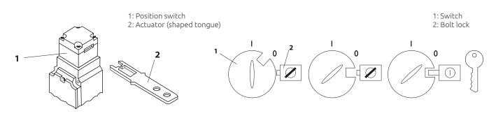
Fig. 9. Type 2 interlocking device - Coded
