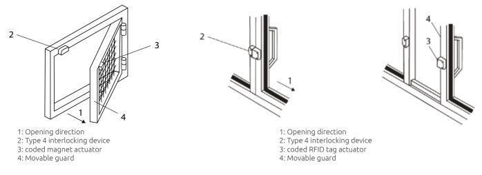
Fig. 11. Type 4 interlocking device - Coded
