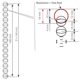
In order to keep in account the dimension of the "Test Rod" (resolution), it is necessary to add 10 mm for each side to the Z dimension.
