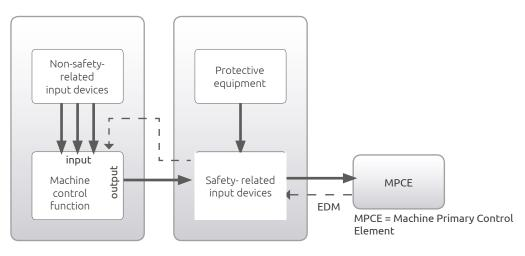
Fig. 21. Machine control and monitoring system (e.g. the PLC) has no safety-related function
