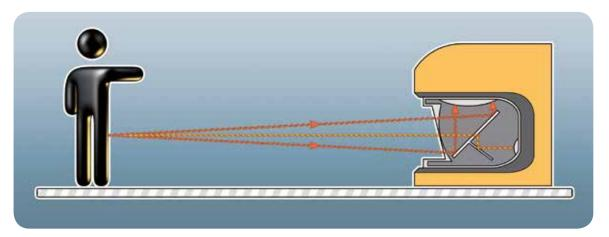
For EN 61496-3, Laser Scanners must be classified in accordance to type 3 or lower safety sensors.
