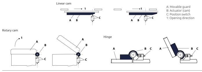
Fig. 8. Type1 interlocking device
