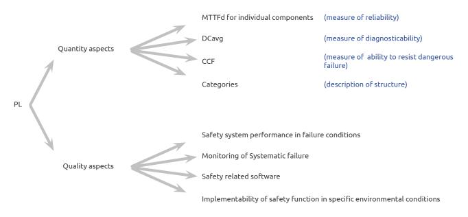
Fig. 3. Mandatory qualitative and quantitative requirements to be met for safe control system design to ISO 13849-1
