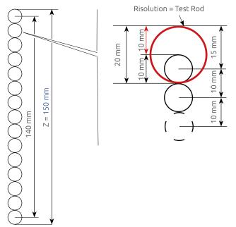
In order to keep in account the dimension of the "Test Rod" (resolution), it is necessary to add 10 mm for each side to the Z dimension.
