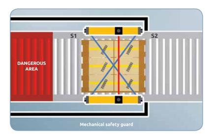
Muting sensor beam intersection shall be positioned the higher up or equal than level of the lower light curtain beam to avoid possible tampering or accidental triggering of Muting.
